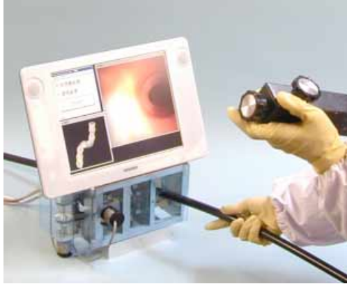
Fig. 15. Total virtual endoscope system with new force display mechanism and large deformable colon model (VES-V)
