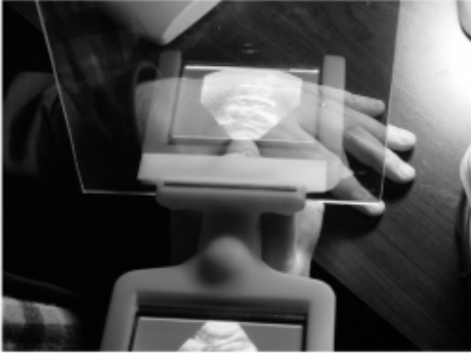
Fig. 3. Photograph from the viewpoint of the operator, showing a scan of the hand using the apparatus in Figure 2. The reflected ultrasound image is merged with the direct visual image.
