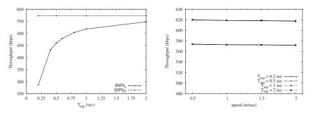
(a) TCP throughputs for the user speed equal to 1 m/s.
