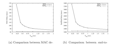
Fig. 5. MAC and end-to-end delays.
