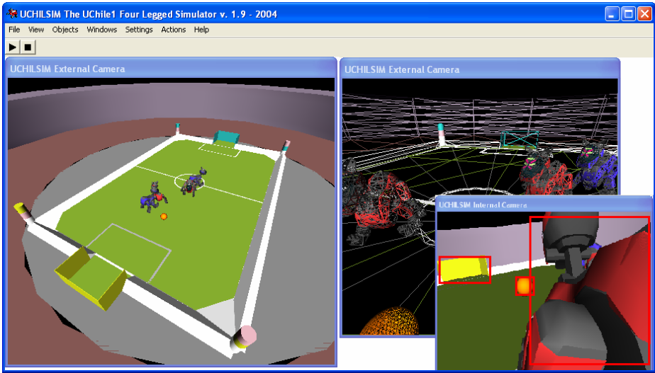
Fig. 1. Illustration of the UCHILSIM software and its user interface. It is possible to observe the display of various viewing options
