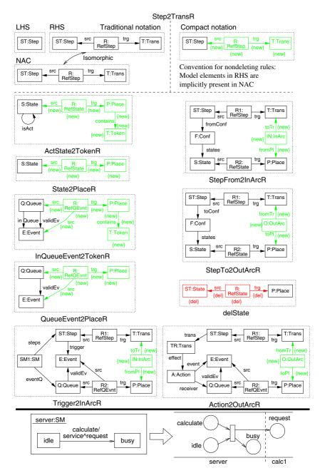
Fig. 2. From state machines to Petri nets
