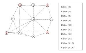
Fig. 3. The connectivity graph of the testbed and its identifying codes. The filled dots denote the positions that transmitters are placed
