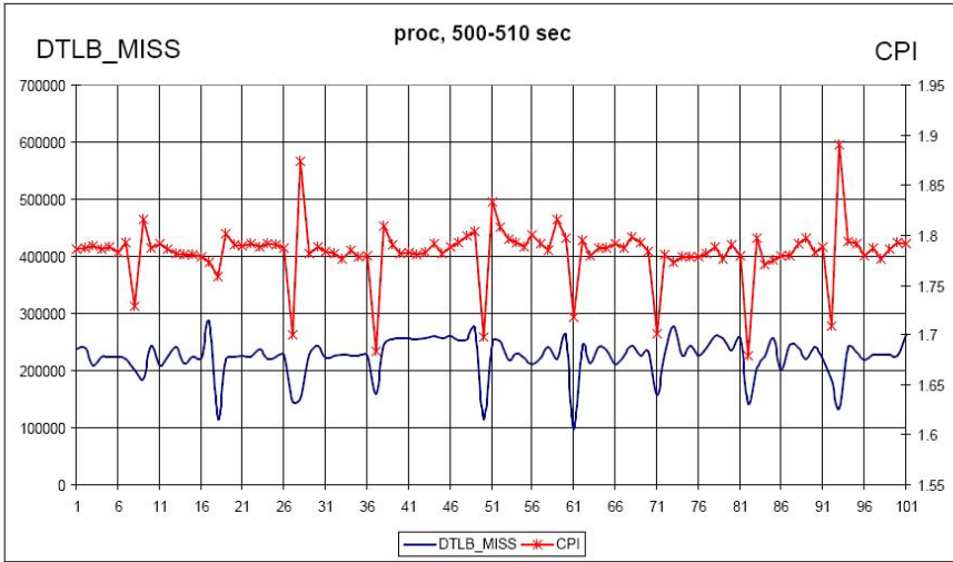
Fig. 2. Correlation between Data TLB (DTLB) Misses and CPI
