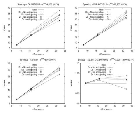
Fig. 2. Speedup and Scaleup Numbers (in relation to 8 processors).
