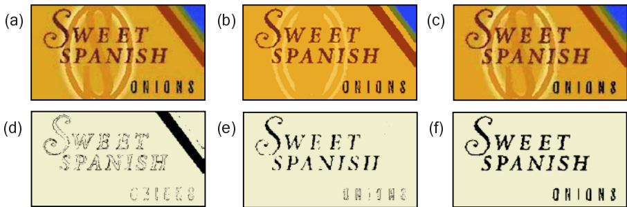
Fig. 2. Test sample : onions advertisement (a) original image, (b) pointer segmentation, (c) pyramid segmentation (d), (e) pointer segmentation color layer 1 and 2, (f) pyramid text extraction.
