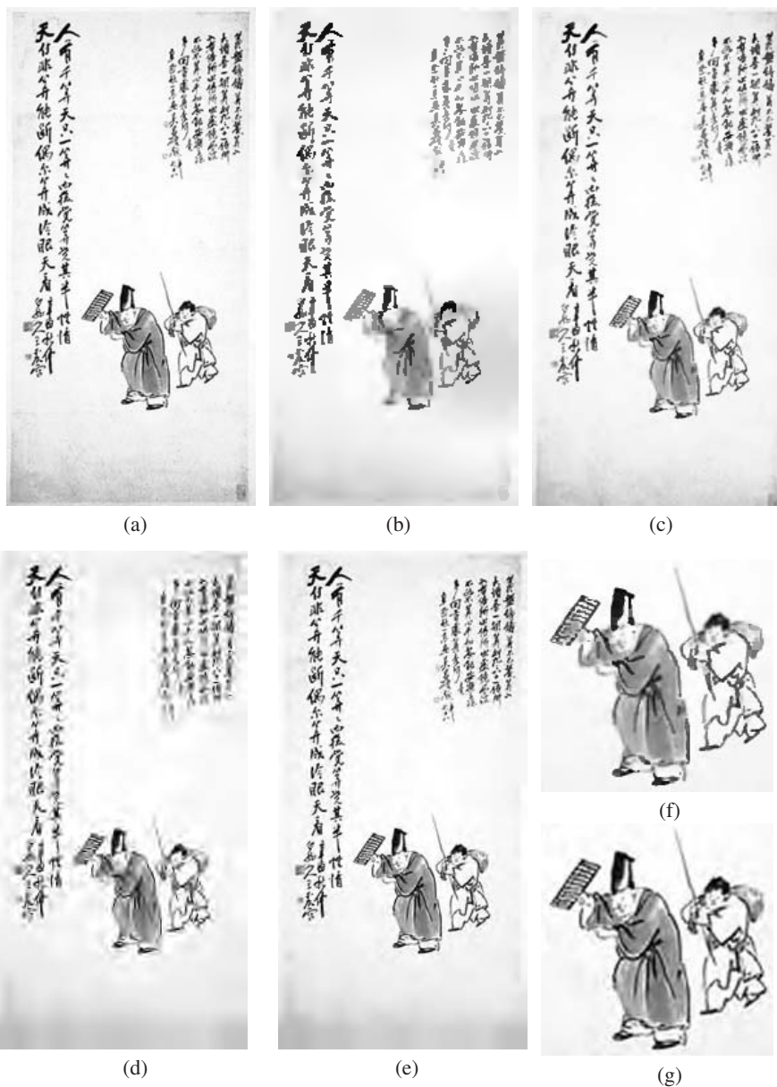
Fig. 6. Chinese ancient art: (a) original image (b) DjVu at 0.028 bpp (c) DjVu at 0.104 bpp (d) SPIHT_roi_max at 0.028 bpp (e) SPIHT_roi_max at 0.104 bpp (f) Zoomed in version of (c) (g) Zoomed in version of (e).
