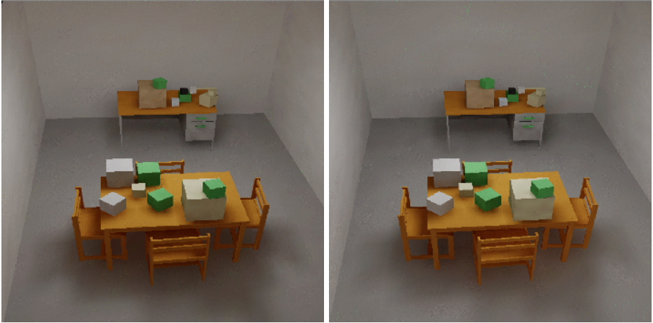
Fig. 3. (left) Frame 17 without reusing paths. 600.000 paths. Time= 70 sec. (right) Frame 17 reusing shooting and gathering paths. 600.000 paths. Time= 11.7 sec. MSE is a bit higher in the second image. Speed-up factor about 4.4
