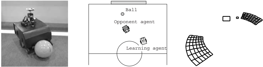
(a) A real robot and a ball (b) Top view of the field (c) Simulated camera image with a omni-directional mirror
