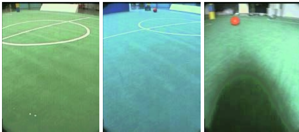
Fig. 2. Examples of the three different lighting conditions used for the experiments. Neon light in Munich in the leftmost picture, pure daylight in Munich in the middle one, and again natural but directed light in our lab in the right image.
