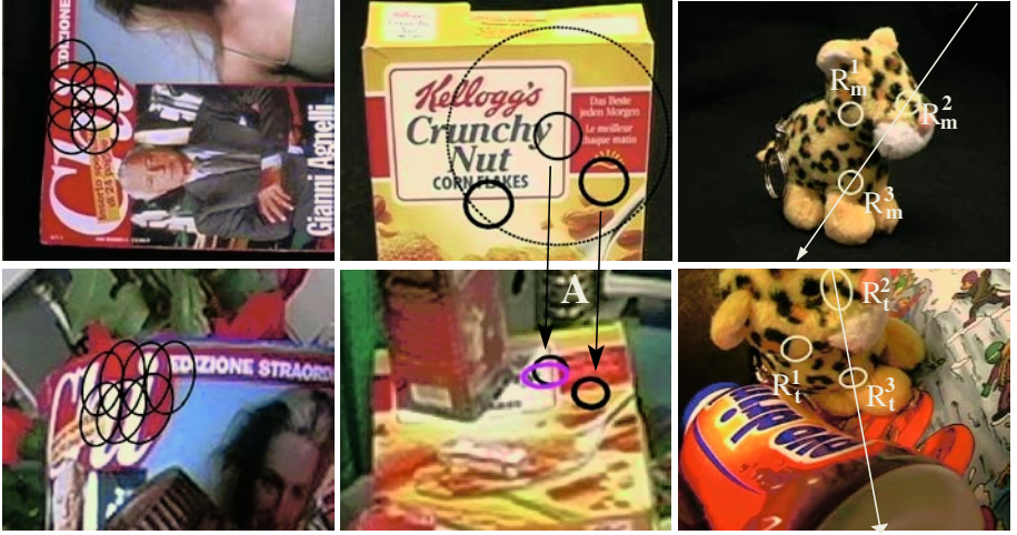
Fig. 3. Left: the regular arrangement of the regions is preserved. Middle: top: a candidate (thin) and 2 of 20 supports (thick) within the large circular area. bottom: the candidate is propagated to the test image using the affine transformation of the support on the right. Refinement adapts the shape to the perspective (brighter). Right: sidedness constraint. R^1 is on the same side of the line in both images
