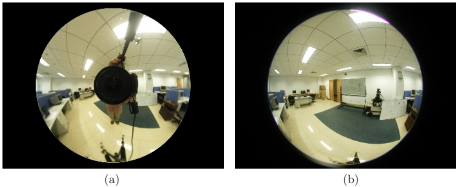
Fig. 1. (a) An image from a central catadioptric camera which is combined a perspective camera with a hyperboloidal mirror, designed by the Center for Machine Perception, Czech Technical University, and its field of view is 217 degrees. (b) An image from a fisheye camera which is a Nikon COOLPIX 990 with FC-E8 fisheye lenses, and its FOV is 183 degrees. The two images are taken in almost same position and direction.
