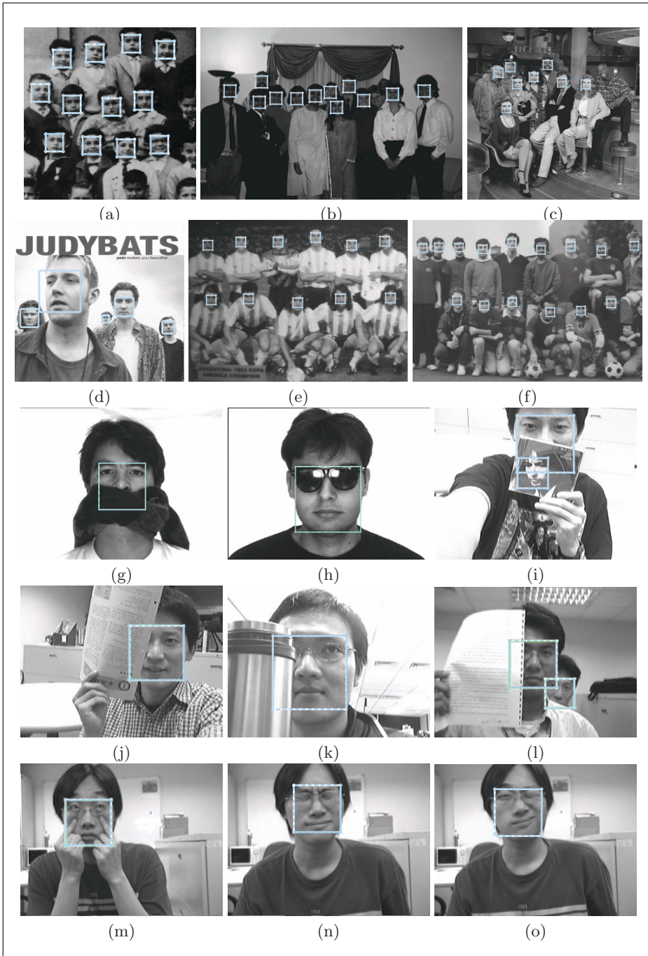
Fig. 4. (a)-(f) Detection results derived by applying our face detector to some of the CMU+MIT data set. (g)-(l) Detection results on several occluded faces. (m)-(o) Detection results for various exaggerated expressions.
