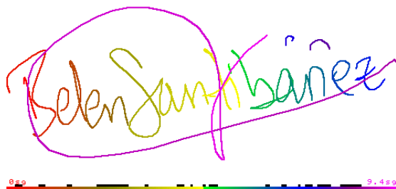
Fig. 1. The digitized signature consists of a sequence of sample points along the signature, captured with a frequency fixed by the acquisition device. Its length is directly proportional to the time of signing, in this example 9.4s. Pen-up symbols occur during the time in black.
