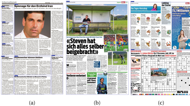
Fig. 3. Good (a) and bad (b) segmentations (blue lines denote crop marks) for realistic pages, depending on the freedom in the layout. Image (c) shows a non-article page that is excluded from automatic segmentation. (Color figure online)
