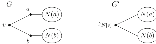
Fig. 2. Illustration of Reduction R.6. Note that, for our argument, it is immaterial whether the edge \{a, b\} is present in G or not.
