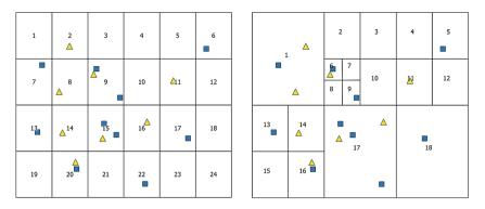
Fig. 1. (a) Regular Grid summarization (b) QuadTree summarization
