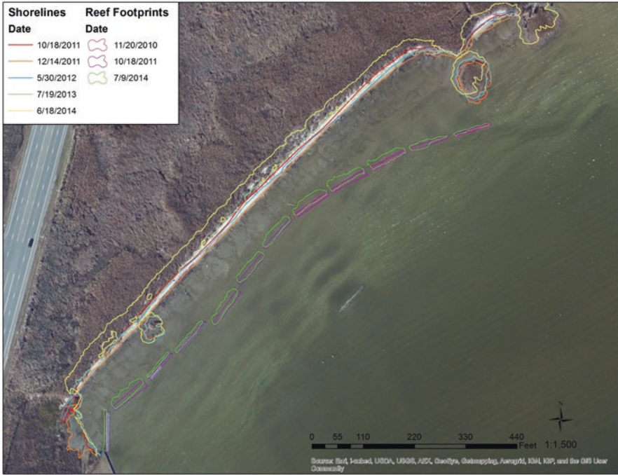
Fig. 13.5 Reef footprints at Helen Wood Park with purple lines showing as built outline in spring 2011. The green line (2014) shows changes after 3 years. The reefs measured ~25 m long and 2–3 m wide with 7.5 m gaps. The two reefs on the left are bagged oyster shells and the reef on the right is made of Reefballs. The second reef on the right is partly made of Reefballs (right side) and partly bagged oyster shells (left side)
