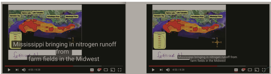
Fig. 2. Picture on left – captions on small personal device display. The viewer increases subtitle size to comfortably read them. The size increase makes the line too long for the screen, and it wraps around, which impacts caption readability. Picture on right – captions on television display. The subtitles are formatted for this resolution and screen by default. The subtitles normally follow caption guidelines to maximize readability for most viewers of the video.
