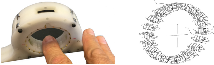
Fig. 5. Left: Reading with the BrailleRing ; Right: Braille-cuboids in a ring-shaped assembly
