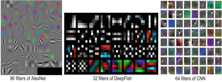
Fig. 4. Visualization of the first convolutional layer filters of AlexNet [10] (96 filters of size 11 \times 11 \times 3 ), DeepFish [4] (32 filters of size 5 \times 5 \times 3 ) and DeepCNN [3] (64 out of 72 filters of size 5 \times 5 \times 3 ) (Color figure online)
