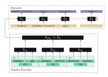
**Fig. 1.** The triple encoder computes a vector representation for each one of the three input triples from the ArticlePlaceholder,  $h_{f_1}$ ,  $h_{f_2}$  and  $h_{f_3}$ . Subsequently, the decoder is initialized using the concatenation of the three vectors,  $[h_{f_1}; h_{f_2}; h_{f_3}]$ . The purple boxes represent the tokens of the generated summary. Each summary starts and ends with the respective start-of-summary *<start>* and end-of-summary *<end>* tokens. (Color figure online)
