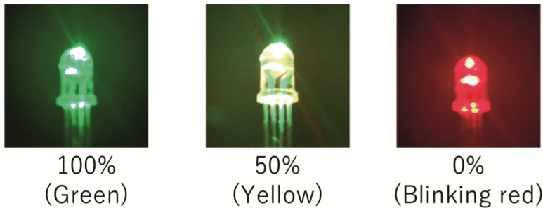
Fig. 4. LED color indicator of the remaining time. (Color figure online)
