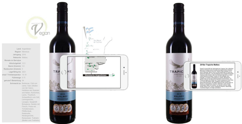
In-Situ Information is anchored in the scene and displayed with respect to the position of the object in this case the bottle of wine.
