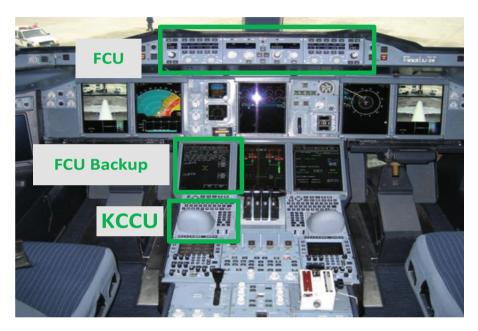
Fig. 1. Two possible means to control flight heading within the A380 interactive cockpit, one using the FCU and the other using the FCU Software application and the KCCU
