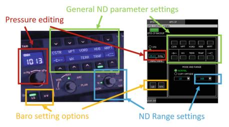
Fig. 3. Baro settings and Navigation Display configuration
