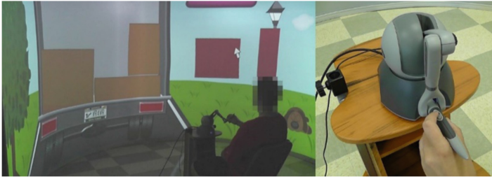
Fig. 3. The haptic device interaction in the VR4VR system. (a) The user controls the cursor in the virtual world by using the haptic device. (b) Haptic device with two buttons on the handle.
