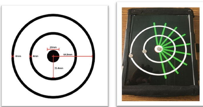
Fig. 5. (Left) Dimensions of the two conditions and their tracing radius, (right) experimental device with circular stickers for two radiuses and tactile markers for start points
