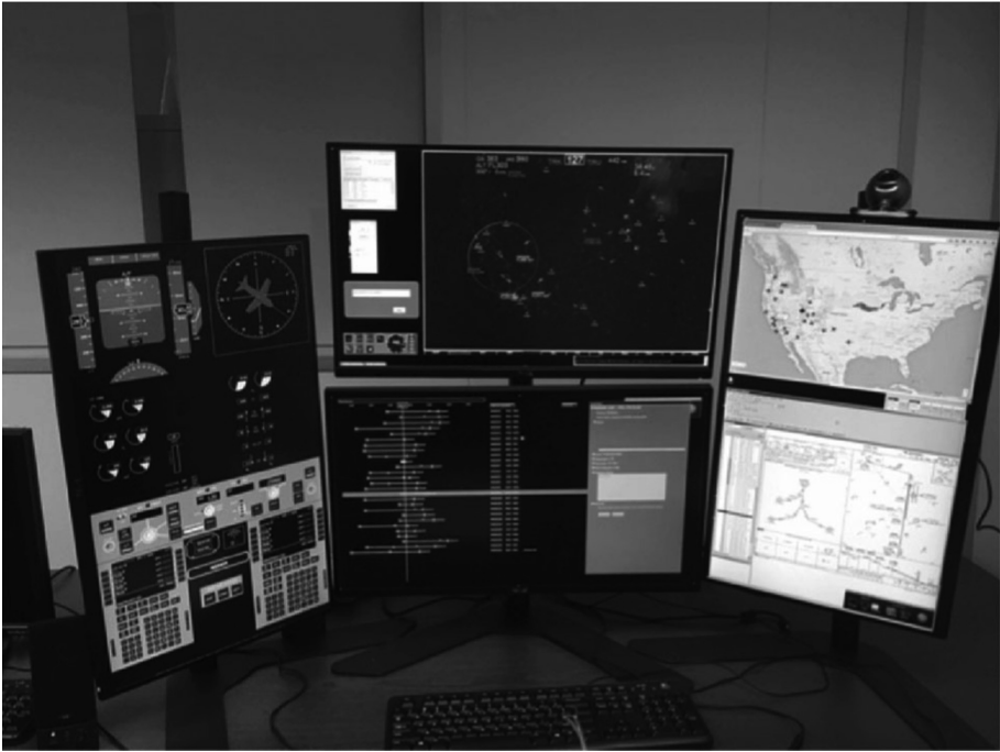
Fig. 4. Build 1 ground station. Bottom center, ACL, augmented with timeline, alerting information; above the ACL is the TSD; to the left is flight controls and displays for the selected aircraft in read-only mode; on the right is CONUS map and charts.
