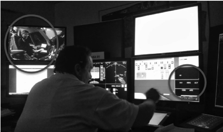
Fig. 2. SPO II ground station. CRM indicators circled on the right and video of the cockpit circled on the left.
