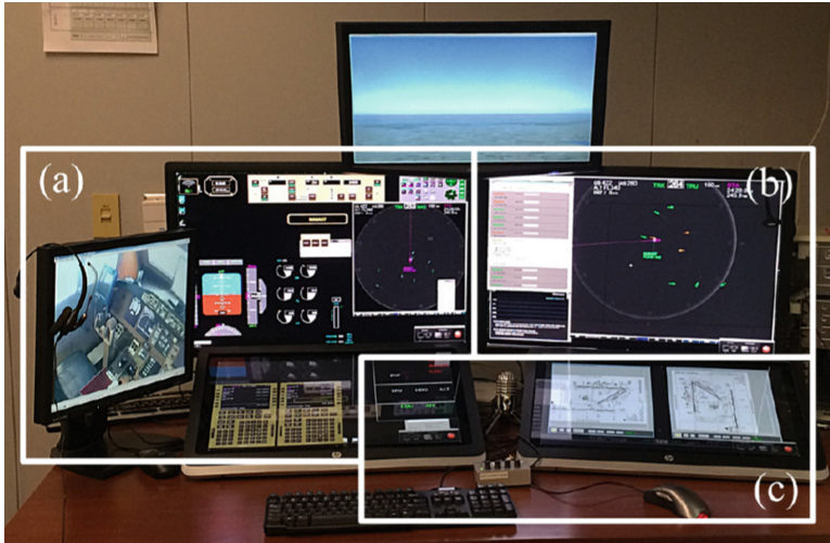
Fig. 3. SPO III dispatch ground station: (a) flight deck displays for the selected aircraft; (b) TSD, ACL with ELP recommendations; and (c) CRM tools and sharable charts.
