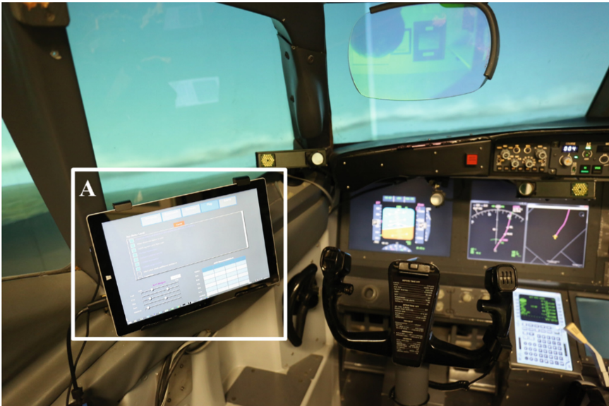
Fig. 8. Flight deck HAT setup: (A) EFB for interacting with HAT features.
