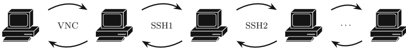
Fig. 3. A diagram of the first evaluation’s setup. The setup comprised twelve virtual machines, coordinating a VNC session and ten SSH remote shell sessions in a series circuit.
