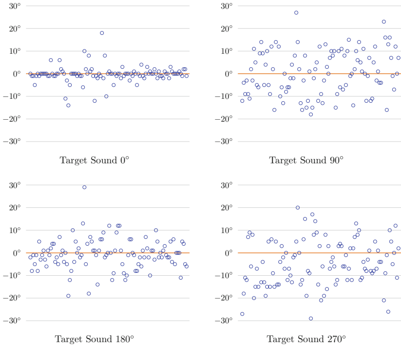
Fig. 4. Scattering of location error around 0, 90, 180, and 270 degree target sound position. The orange line represents the target sound position. The blue circles mark participants' determined sound locations. (Color figure online)
