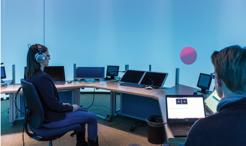
Fig. 1. The 360-degree tower simulator during the experiment. The participant wears a headphone with an attached head tracker to control the sound position and the digital red ball on the wall. (Color figure online)
