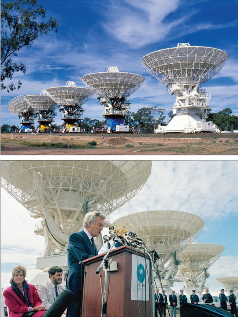
Fig. 5.16 (above) Five of the six 22 m dishes making up the ATCA. The sixth dish is 3 km to the west. (below) The Australia Telescope was officially opened by Prime Minister Bob Hawke in September 1988, as part of Australia's Bicentennial celebrations. At left are Hazel Hawke and science minister Barry Jones (courtesy: CRAIA)
