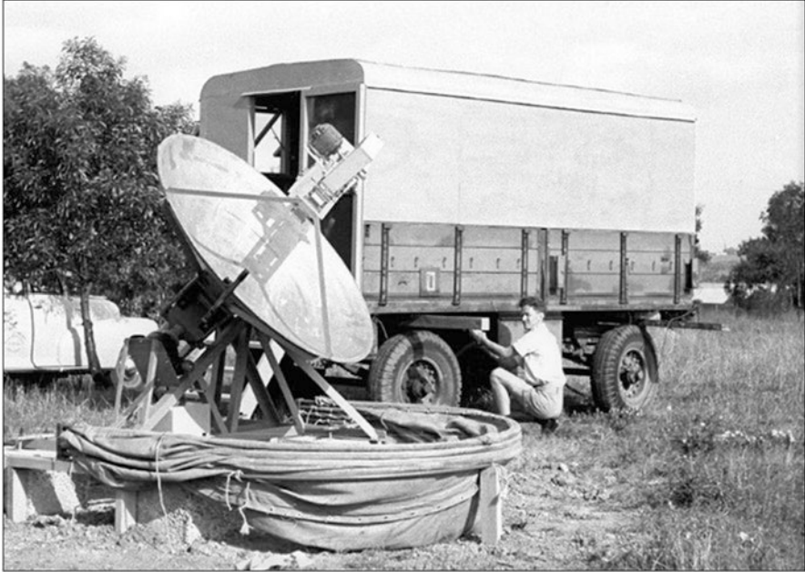
Fig. 2.38 The 1.7 m equatorially-mounted antenna was used in the late 1940s and early 1950s for solar monitoring at 3000 MHz, shown here with preparations underway for the November 1948 solar eclipse (courtesy: CRAIA)
