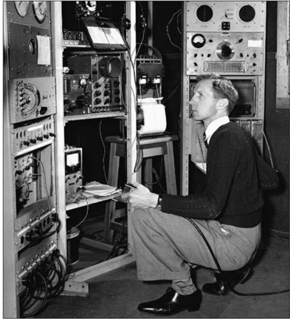
Fig. 2.44 The 4-channel hydrogen-line receiver. Taking readings is Brian Robinson who joined the H-line team in 1953 (courtesy: CRAIA)
