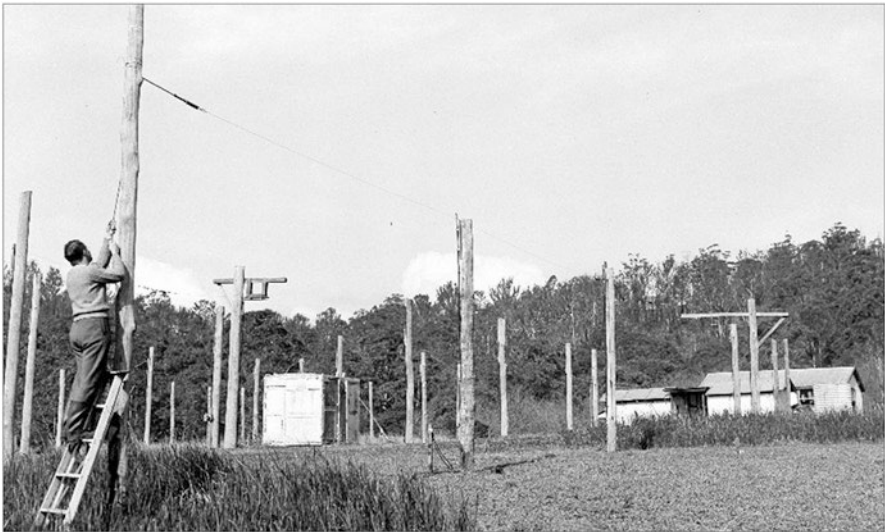
Fig. 2.30 Some of the 9.15 MHz aerials at Hornsby Valley used in the low frequency sky survey centred on declination -32^\circ (courtesy: CRAIA)
