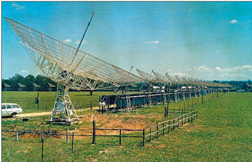
Fig. 1.25 View looking west along the E–W arm of the Fleurs Synthesis Telescope. In the foreground is one of the new 13.7 m antennas, and beyond it the smaller dishes belonging to the original Chris Cross (courtesy: CRAIA)
