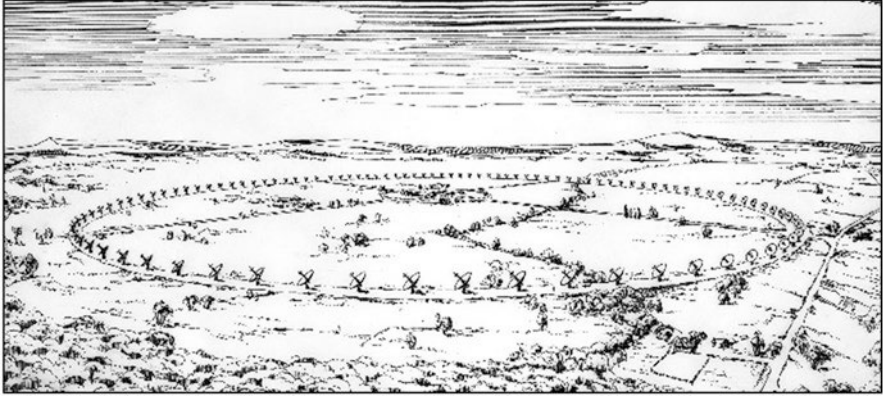
Fig. 1.23 Sketch of Paul Wild's 96-element solar Radioheliograph (courtesy: CRAIA)
