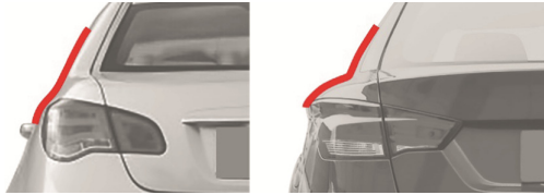
Fig. 9. Relation features of side window and the side of body in rear view
