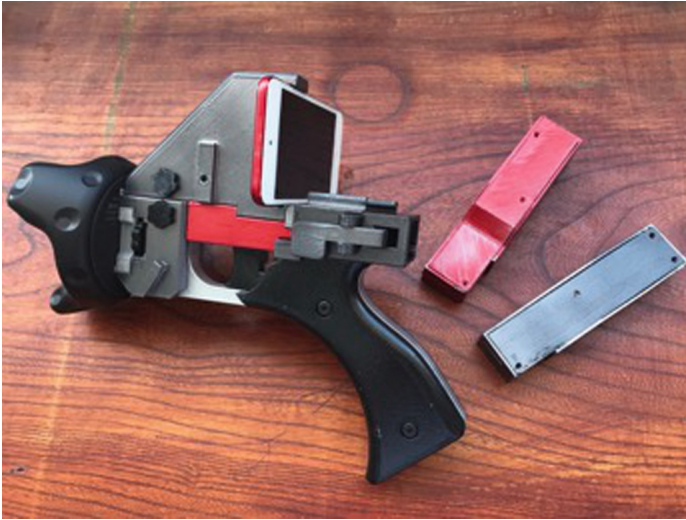
Fig. 8. Current VAIR Gun and magazines. (Press the lever on the left rear side to release the magazine. By pushing in a magazine from behind, it is automatically locked and loaded with bullets.)
