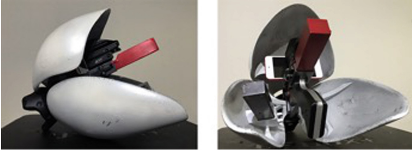
Fig. 9. Fully equipped VAIR Gun. (Spare magazines can be stocked inside the cowl.)
