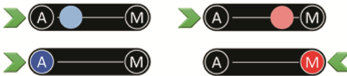
Fig. 4. Examples of the actuator display for CA, UA and PA conditions which were visually identical, differing only in the algorithm used to control their behavior. In the top left the automation is in control and the output of the control algorithm is leaning towards automatic control. In the top, right the automation is also in control, but the controller is leaning towards manual control. In the bottom left the automation is in control, and the controller is suggesting that this state be continued. In the bottom, right, the participant is in control and the controller is suggesting that they remain in control. (Color figure online)
