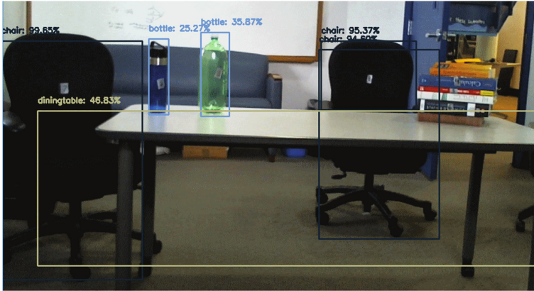
Fig. 2. Object detection and localization with a Single Shot MultiBox Detector
