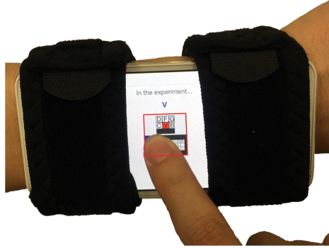
Fig. 3. Smartphone attached in a landscape orientation with respect to the non-dominant hand.
