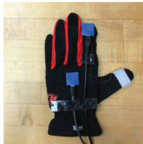
Fig. 4. The glove with IMUs attached on the back of the hand and on the tip of index finger
