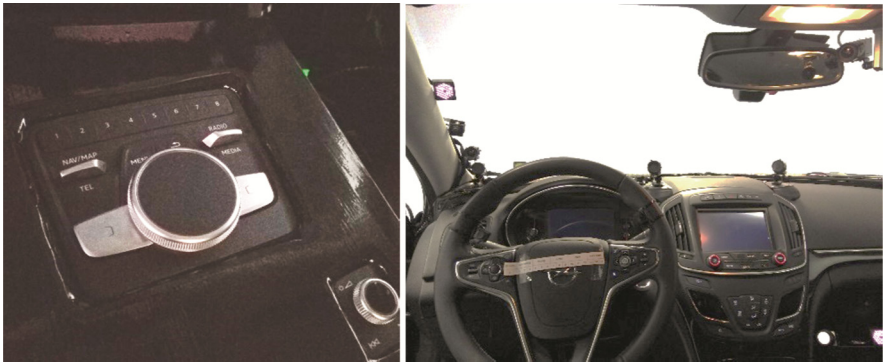
Fig. 1. Simulator setup; left: rotary control knob; right: eyetracking cameras
