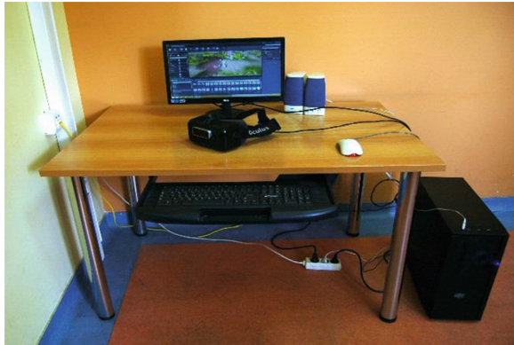
Fig. 2. The equipment needed for our platform. We used the most accessible VR technology in order to create a low-cost platform, easily reachable by patients. They wear an Oculus Rift headset, have their hands tracked by a LeapMotion controller and they can hear the music through a set of desktop speakers.
