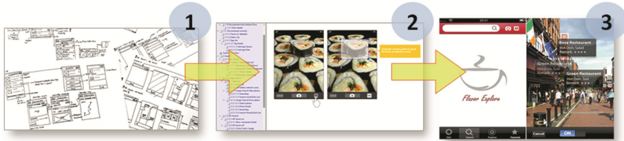
Fig. 2. (1) Wireframes of user interfaces, (2) the interactive HTML prototype created with axure, and (3) high-fidelity prototype created with Adobe Flash Catalyst.
