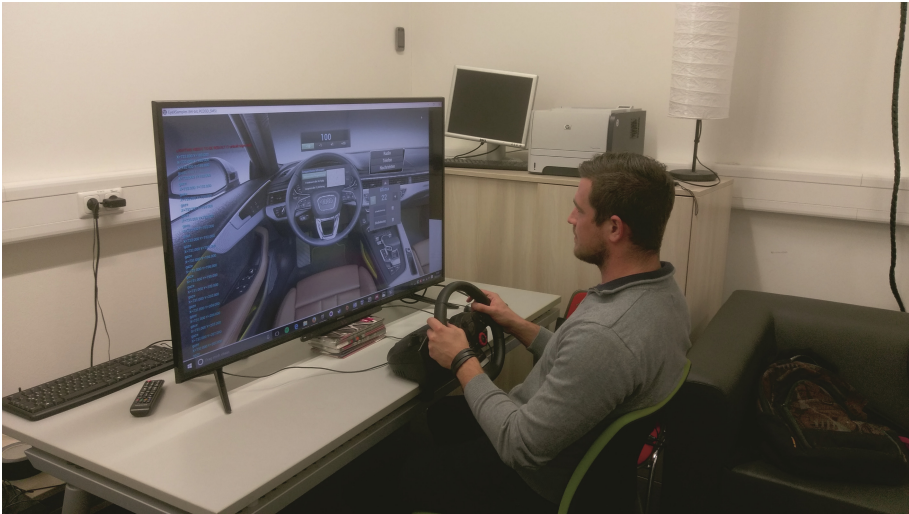
Fig. 1. Test setup in front of a 48" TV with a steering wheel and an eye tracker beneath the TV.
