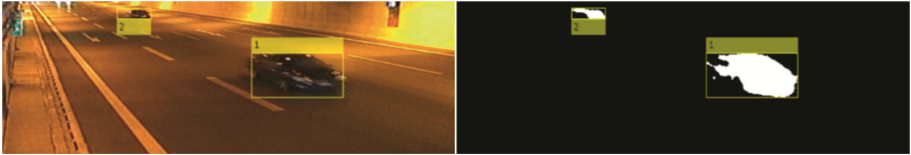
Fig. 8. Blob tracking based on foreground detection
