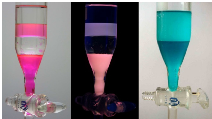
Fig. 7 A picture of a four-phase solvent system (left and centre) composed of (top to bottom) hexane, trihexyltetradecylphosphonium bis((trifluoromethyl)sulfonyl)amide ( [\text{P}_{6,6,6,14}][\text{NTf}_2] ), water and 1-ethyl-3-methylimidazium bis((trifluoromethyl)sulfonyl)amide ( [\text{C}_2\text{mim}][\text{NTf}_2] ), using eosin Y as a luminescent dye which is soluble in the two ionic liquid-containing phases. The central photograph is of a system illuminated with 254-nm UV light. Also shown is a two-phase solvent system (right) of [\text{P}_{6,6,6,14}]\text{Cl} (upper phase) and [\text{C}_2\text{mim}]\text{Cl} (lower phase) with cobalt(II) Cl as the blue chromophore. In the two blue phases, the complex is tetracobaltate(II) [40]
