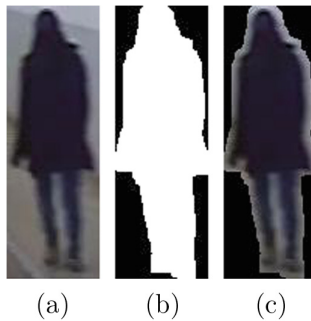
Fig. 8. The multiplication of detected person with its mask, (a) Detected person, (b) Mask of detected person and (c) Results of multiplication
