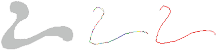
Fig. 1. From left to right, an object, its skeleton (different colors denote different distance values), and the vertices (black) resulting in the skeleton after polygonal approximation in 3D. (Color figure online)
