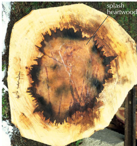
6.142 "Splash heartwood" (German "Spritzkern") in Fagus sylvatica is a sign of bacterial infections.
