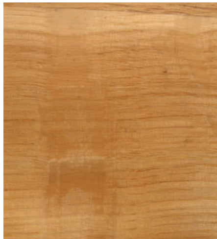
6.154 The radial cutting direction shows the structure of the rays in parquet flooring of Quercus sp.
