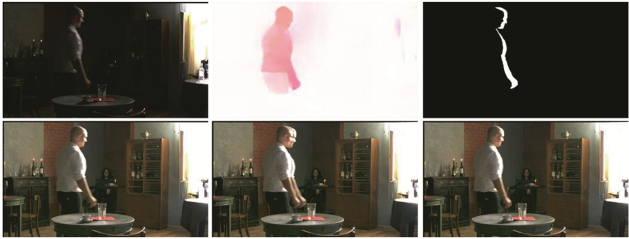
Fig. 4. Example of occlusion fixing process. ( Left Column ): current reference frame ( Left-Top ) and its next frame ( Left-Bottom ). ( Middle-Top ): optical flow estimated by our CNN model from current frame to its next frame. ( Middle-Bottom ): directly reverse warped result using the flow, which shows ghosting at regions of occlusion. ( Right-Top ): occlusion map extracted from optical flow map. ( Right-Bottom ): warped LDR result after our occlusion fixing process.
